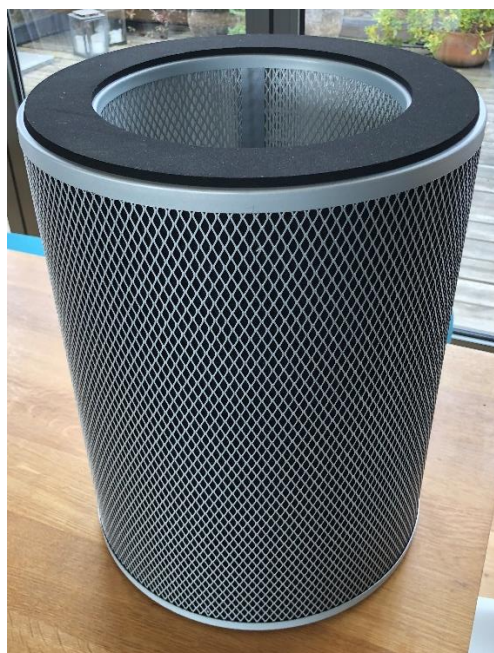
Figure 1: Left) Device under test – Rensair. Right) HEPA-filter removed from device.
